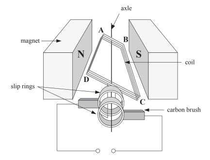
The diagram above shows a wind-powered generator in a yacht. It comprises a rectangular coil of wire that is rotated in a magnetic field.
