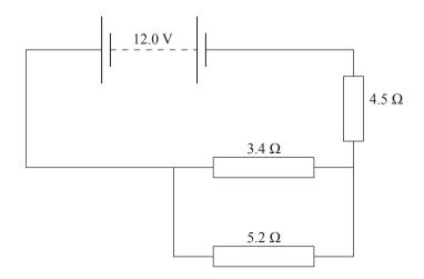
(a) How much energy does the battery give to each Coulomb of charge?
